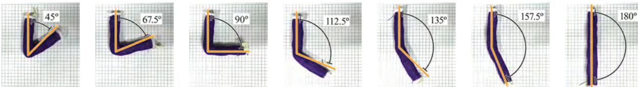
Figure 6.13: A series of bent tubes fabricated using the incremental remeshing algorithm. Short-rows are automatically produced by the procedure and accurately generate the bending angle.
