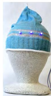
Figure 2.13: Using conductive yarn for LEDs
