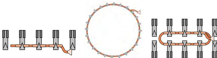
Figure 2.5: Different needle layouts for different styles of machines. (Left) A single linear layout for flat knitting, (Middle) Circular layout for seamless tubular knitting, (Right) Two bed layout for whole garment knitting
