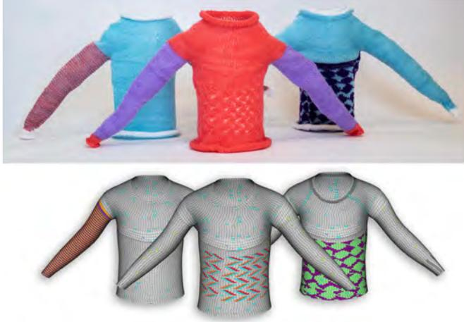
Editing can be used to align decreases and increases for the desired aesthetic effect. The automatic remeshing often distributes increases and decreases to accurately match the 3D geometry but aligned decreases can generate a more pleasing appearance for garments.
